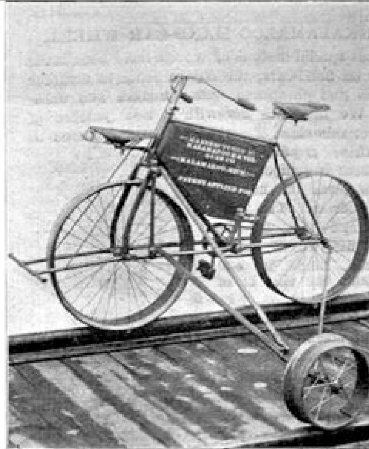
Fig. 2. New Track Velocipede with Toolbox and Extra Seat Attached.
